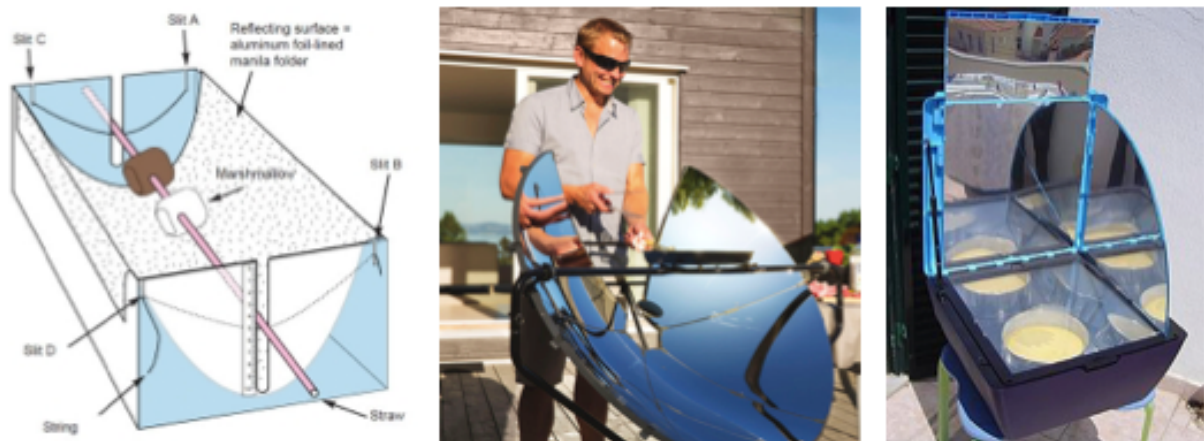
Figure 5: Solar Cookers a) Concentrating Sunlight [12] b) Converting Light Energy into Heat Energy [13], c) Trapping Heat Energy [14]
